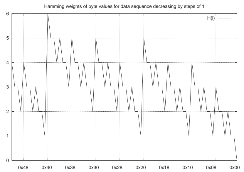
Fig. 8. Computed Hamming weights for data ranging from 76 down to 0, decreasing by steps of 1.
